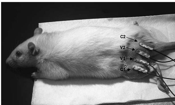
Fig. 2. Experimental set-up for surface recordings. C1 and C2 are the current-injecting electrodes and V1 and V2 are the voltage electrodes.
