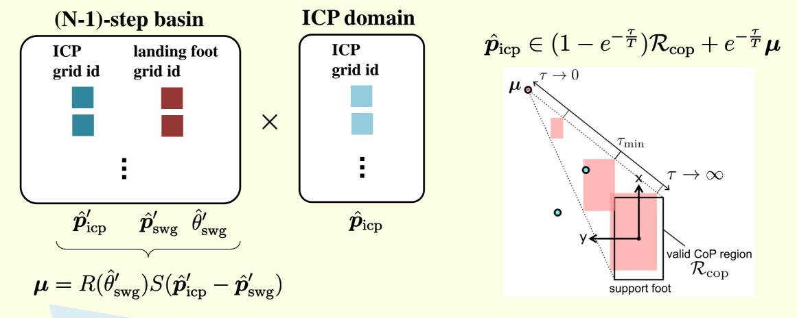
Position of ICP at landing (expressed in the current support-foot coordinate)
