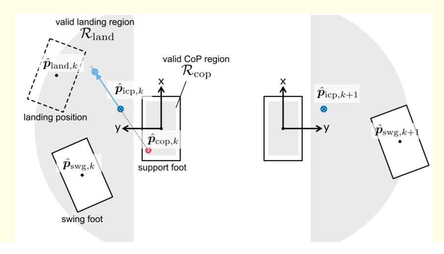
Step duration is lower-bounded by the travel distance of the swing foot (cannot step too quick)
