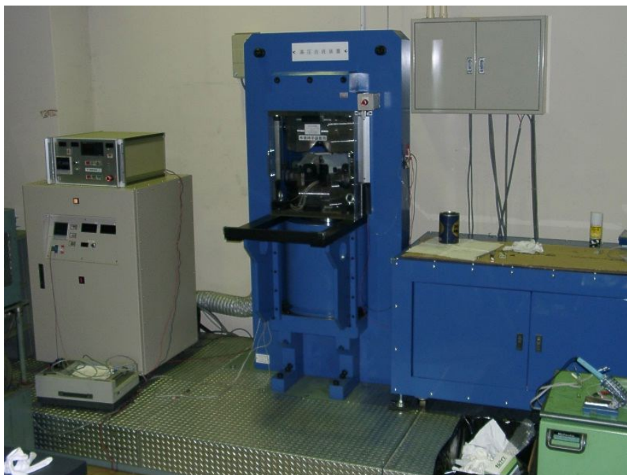
Figure 1: Photograph of a 700 ton cubic-anvil apparatus in our laboratory.
