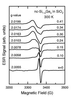
FIG. 3. ESR derivative spectra of nc-Si<sub>1-x</sub>Ge<sub>x</sub> dispersed in SiO<sub>2</sub> thin films at room temperature. Ge concentration is changed from 0 to 0.41.
