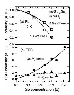
FIG. 2. (a) PL intensities of the 1.4 and 0.9 eV peaks at 10 K, and (b) the integrated intensities of the ESR signals from Si and Ge  $P_b$  centers as a function of Ge concentration.
