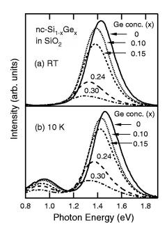
FIG. 1. PL from nc-Si<sub>1-x</sub>Ge<sub>x</sub> dispersed in SiO<sub>2</sub> thin films (a) at room temperature and (b) at 10 K. Ge concentration is changed from 0 to 0.30.
