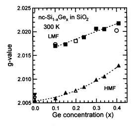
FIG. 4. *g* values of the HMF ( $\blacktriangle$ ) and LMF ( $\blacksquare$ ) signals as a function of Ge concentration. The data for Si  $P_b$  centers [ $\triangle$  (Ref. 12),  $\nabla$  (Ref. 16), and  $\blacktriangledown$  (Ref. 19)] and Ge  $P_b$  centers [ $\Box$  (Ref. 12), and  $\bigcirc$  (Ref. 13)] are also plotted. The broken curves are drawn to guide the eyes.
