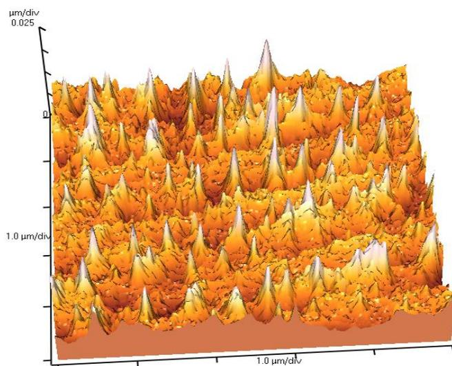
3D AFM image of Ge surface irradiated by Nd:YAG laser at intensity  $6.0 \text{ MW/cm}^2$ .
